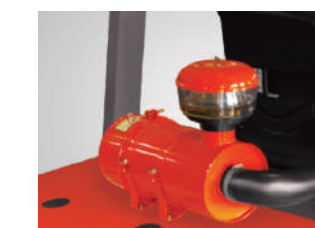
Pre-cleaner engine air intake
